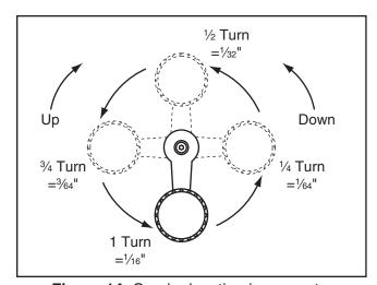
Figure 14. Crank elevation increments.
